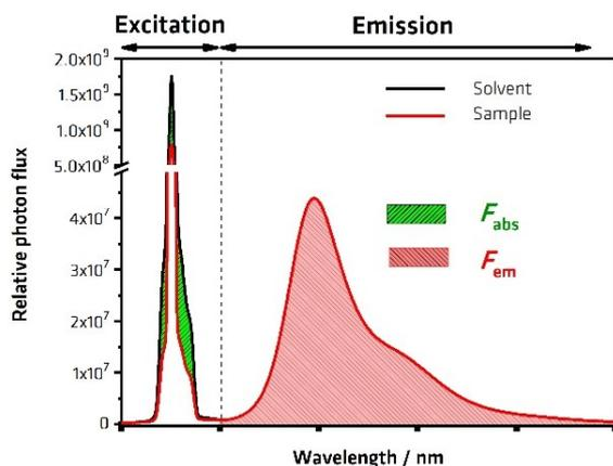
**Fig. 2** Scheme of the determination of the relative photon flux emitted from the sample (red area) and the relative absorbed photon flux (green area) measured with an integrating sphere setup.
